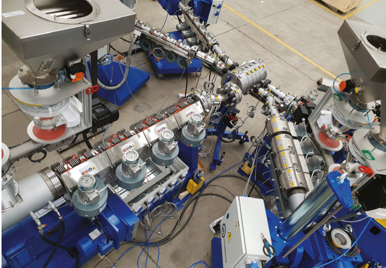
Above: A European pipe producer is using Tecnomatic's Athena die head to make five-layer PE-RT and PEX pipe
