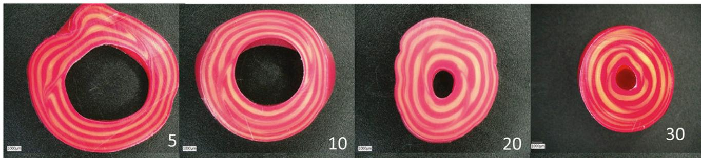
**Above: Case Western has developed a die that could apply 'layer multiplication' to pipes**
